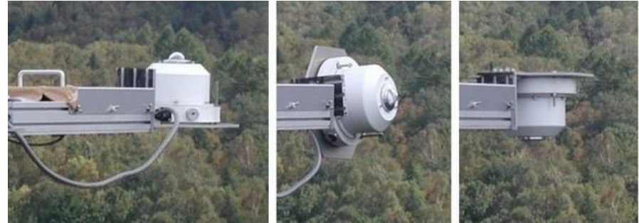
HSSR (Hemi Spherical Spectro-Radiometer; MS700 spectrum radiometer (EKO) + rotater (Hayasaka Rikoh)
